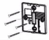
Focus the drilled hole on the wall and fix the back cover on the wall by screws.
