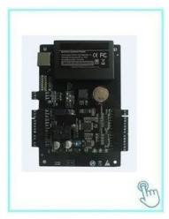
$\begin{array}{l} \textbf{C3-100/200/400} \\ \textbf{Access control panel for 1/2/4 doors} \end{array}$
