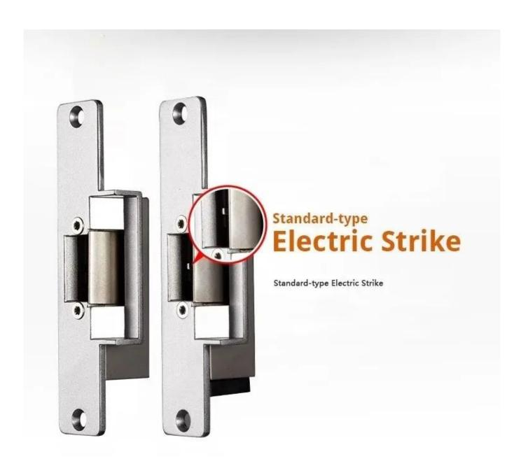
ACM-Y138 NO/NC is the electric strike with long faceplate. It has two modes: A fail safe electric strike needs power to keep it locked. A fail secure electric strike stays locked even without power. Electric strikes come in many varieties.
