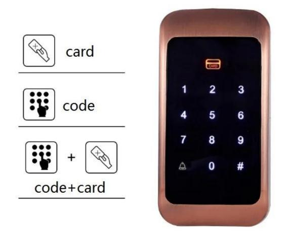
This reader can work work as a stand alone RFID access control reader ,also it can work as a normal wiegand 26 reader which can connect to the control board to control the door . Following is the wire connection of the 2 working mode .
