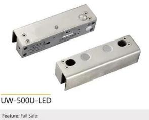
Feature: Fail Safe Face Plate: 185Lx25.7Wx37H(mm) Bolt: 16(length)x12.7(diameter)(mm) Voltage: DC12V Start Current: 960mA
