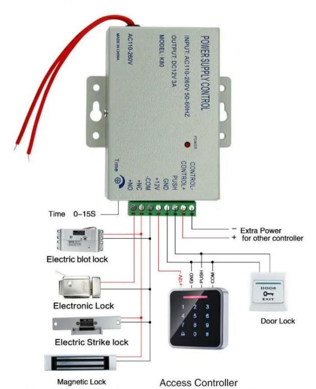
Attention when electronically contriled lock must be transferred to 0seconds delay,to prevent burning of electric lock.
