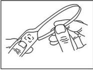
**Insert strap into locking chamber**
