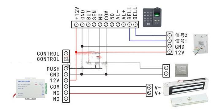
With Feedback Function Magnetic Lock Connection Diagram
