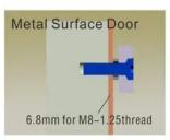
Inside:Drill a hole diameter is 8mm folding the plastic straight pin
