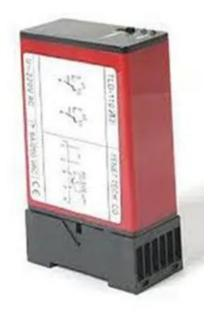
Loop detectors are used wherever vehicles have to be detected. Like monitoring and safe guarding access ways for counting vehicles. The output signal can be used for controlling door and gate drive mechanisms, road barriers, controlling traffic light systems in car parks or activating card dispensers in car parks.
