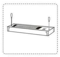
2.Use a screwdriver to unscrew the anti-removal screws.
