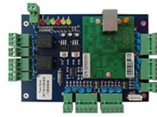
Network TCP/IP Access Control Board
