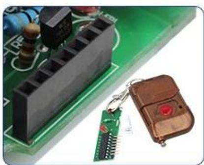
The access control power board slot design can insert the remote control module into the slot and unlock it with one button.
