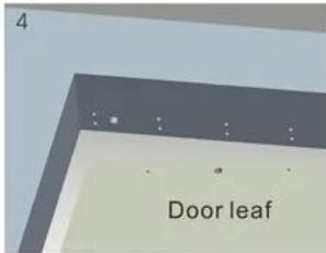
4 Drill holes based on the marked positions.
