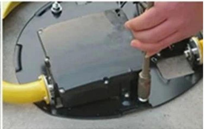
4. Tighten the screws with a suitable wrench
