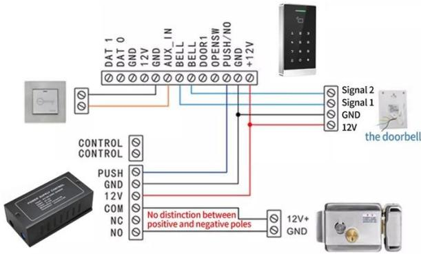
Note: The power controller needs to be connected to 220V, and other accessories can be connected with a network cable
