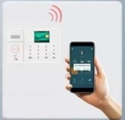
⑥ The main panel will inform user by call after receive sensor signal
