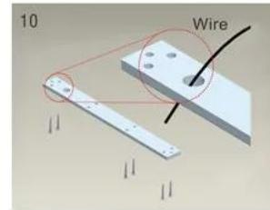
10 Fix the mounting plate on the door frame according to the holes drilled earlier.
