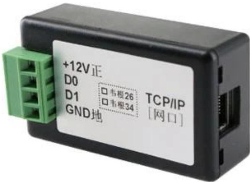
WG to TCP Converter diagram
