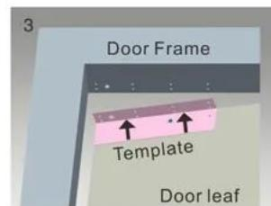
Mark screw positions of armature plate and magnetic lock on door leaf and door frame respectively.
