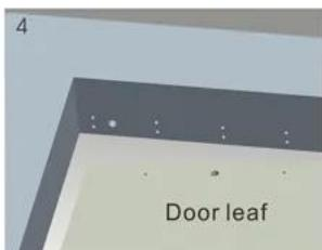
Drill holes based on the marked positions.
