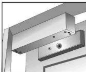
Amature plate installation
