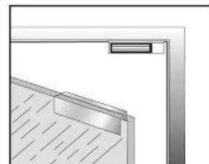
UL bracket installation
