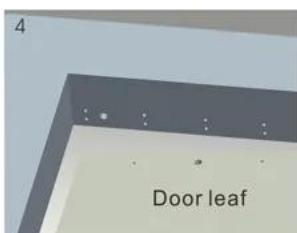
Drill holes based on the marked positions.
