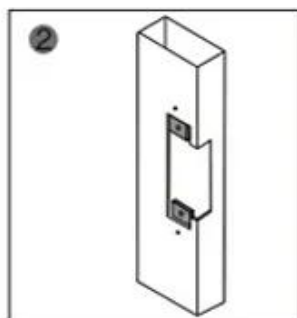
2 Insert extension plate
