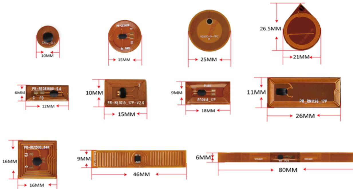
Flexible circuit board (Flexible PCB): Referred to as "flexible board", FPCB features: Can add anti-metal layer and adhesive, suitable for bending and use, light and thin, foldable, small pitch, multi-pin, small volume, high integration, multi-contact, etc. It is suitable for the design of custom labels, including special requirements for the shape.
