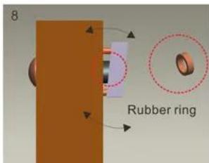
Place the rubber ring between armature plate and door leaf.
