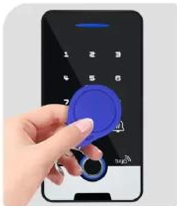
IC card swiping to open the door
