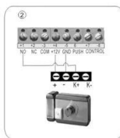
Attention! then electronically controlled lock must be transferred to 0 seconds delay, to prevent burning of electric locks.
