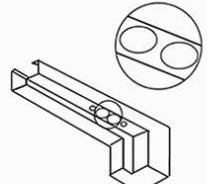
3. Use a hole opener to open the lock hole
