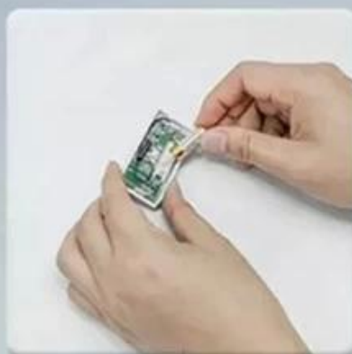
② install 23A 12V battery
